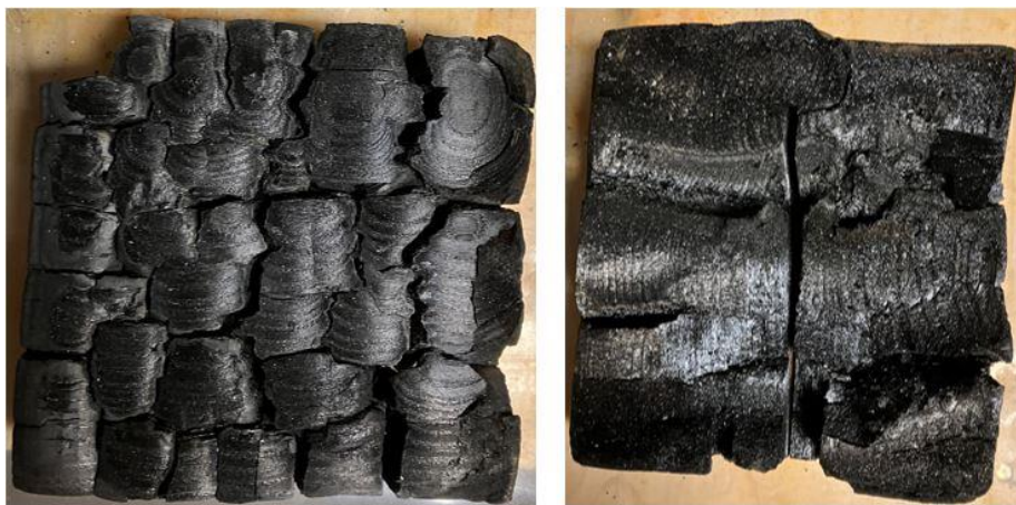
Figure 4: Sample images of the char produced by the hardwoods (left) and softwoods (right) when exposed to 50 kW/m 2 for 30 minutes (author’s photos)
