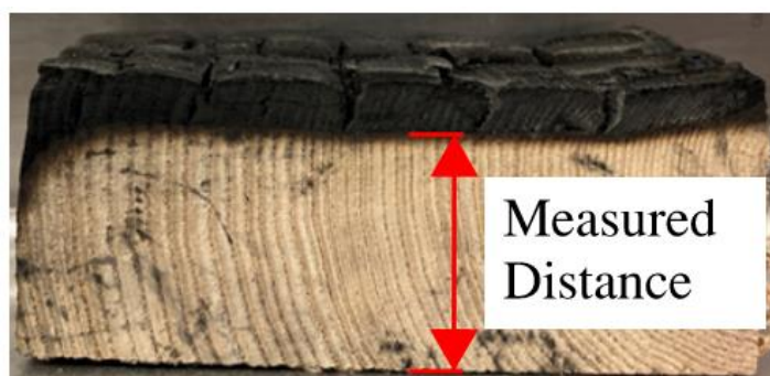
Figure 3: Cross-section of a sample with dimension indicating where uncharred depth is measured
