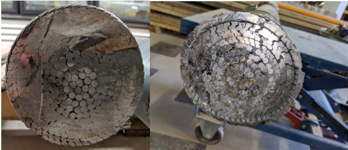
Figure 3. Cross-section view of L-GS-100A (left) and L-GS-100B (right) experimental sample, taken after experimental testing
