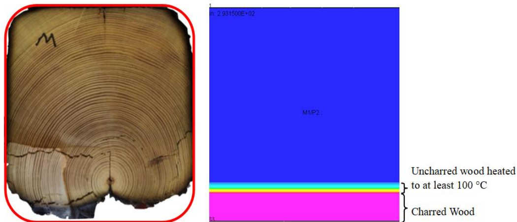
Figure 4: Comparison of the charred member and numerical model of a) the Glulam members and b) the heritage members
