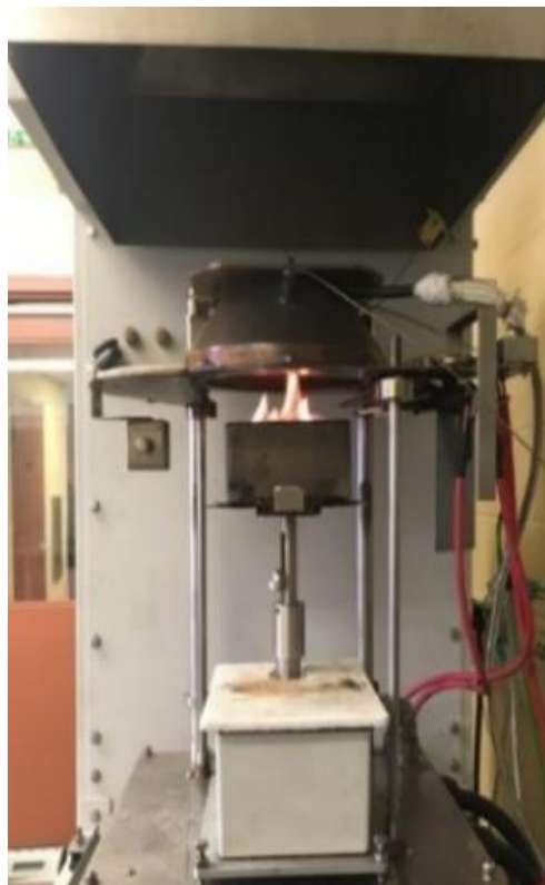
Figure 7. Cone calorimeter test setup.
