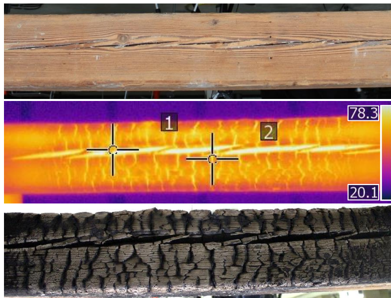
Figure 8. Side A crack progression before (top) and after fire (middle and bottom) on Heritage 2 (identifiable markings were recorded temperature markers and scale is in °C).
