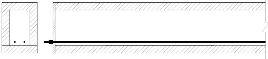
Figure 2.6: Schematic of typical PT timber beam cross-section showing built up wood webs and flanges and high-strength steel tendons, along with section cut through beam length showing tendon anchorage
