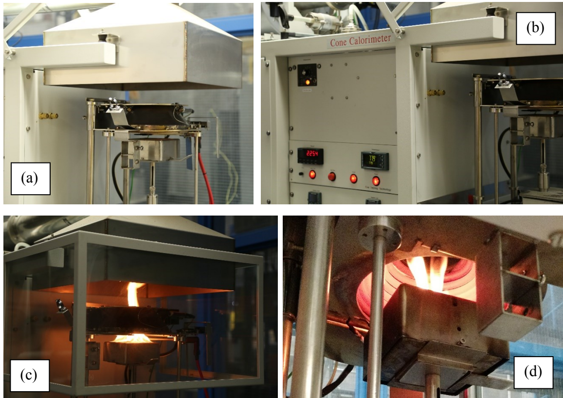
Figure 4.2: Cone Calorimeter apparatus showing (a) the hood used to collect test emissions for calorimetry, (b) the apparatus display, (c) a specimen during heating with the shield deployed and (d) the conical heating element during heating
