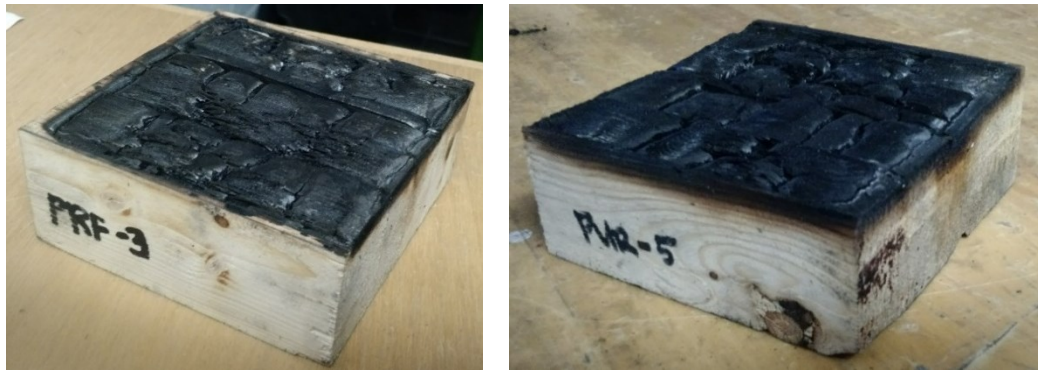
Figure 4.8: Samples after burning exposed at 50 kW/m 2 ; on the left a PRF sample exposed for 3 minutes and on the right a PUR sample exposed for 6 minutes
