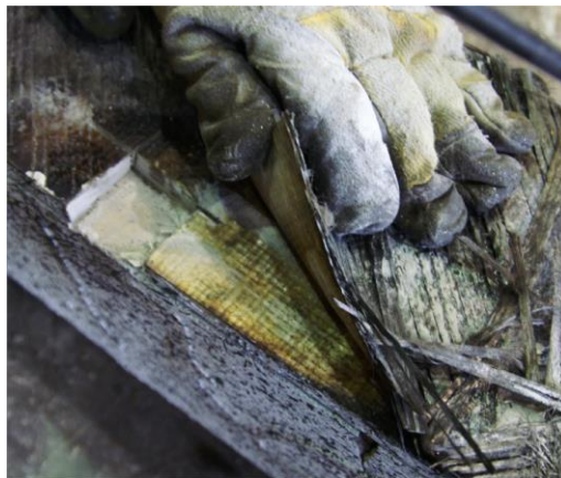
Figure 4.23. Delaminated pyrolysis/char layer on GFRP base plate soffit.
