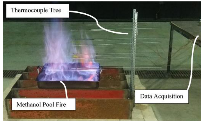
Figure 5.4. Typical fire characterization test configuration.
