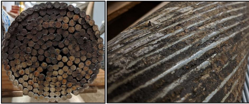
Figure 5.2. Cross-section and surface view of cable S-GS-114 demonstrating a rope closing level application of ANTICORIT WRCP J207 blocking agent.
