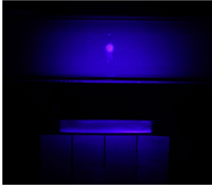
Figure 4. 11: Photograph captured for DIC analysis at the centre span, with the flame filtered out using narrow spectrum illumination.
