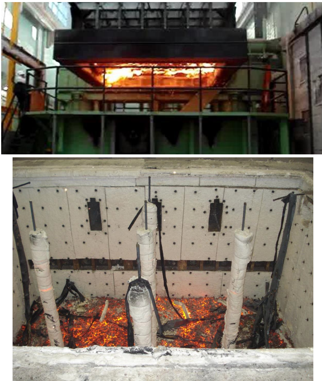
Figure 1. Standard Fire Resistance Test of a Wooden Floor (at test conclusion - author's photos).
