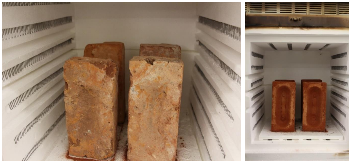
Figure 5.3. Brick configuration in the furnace (1840s and new (2010s) bricks).
