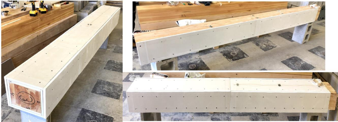
Figure 4.6 Encapsulation procedure of a column protected by three layers of gypsum board, clockwise from top right: first layer installation in progress, first layer complete, third layer complete.
