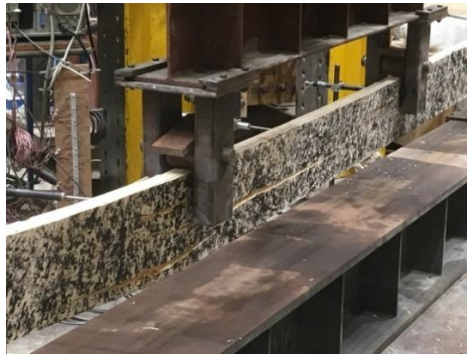
Figure 6.3. Failure mode of a Glulam undamaged control beam.
