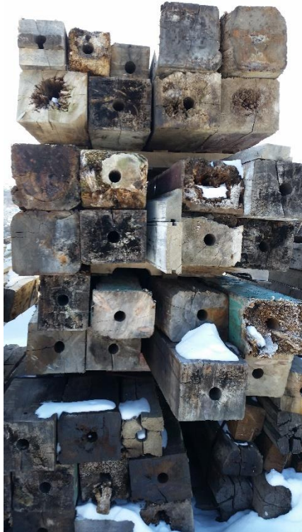
Figure C.3 Improper storage of heritage timber materials (by permission).
