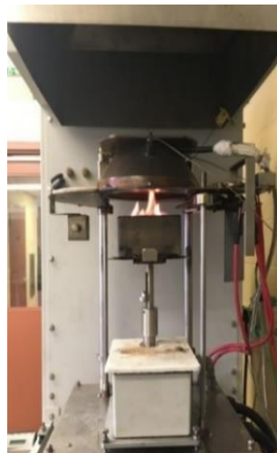
Figure C.6 Cone calorimeter test setup.
