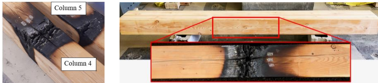
Figure 4.21 (left) Post-test condition of Columns 4 and 5 (right) post-fire cracking of Column 4.
