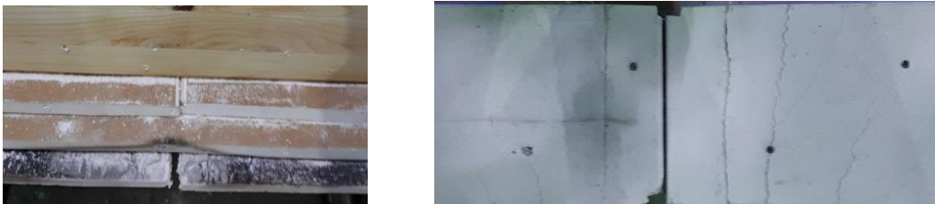
Figure 4.18 Post-fire 'seam' opening in Column 3.
