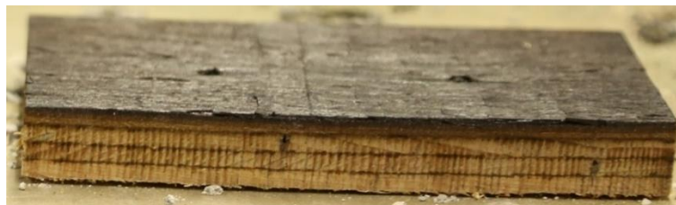
Figure 3.11 Degradation process beginning on the timber, seen after removal of the iron plate.
