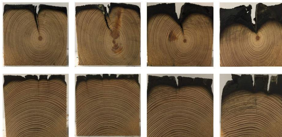
Figure C.13 Char depth of cracked (top) and solid (bottom) timber samples at various exposure durations.
