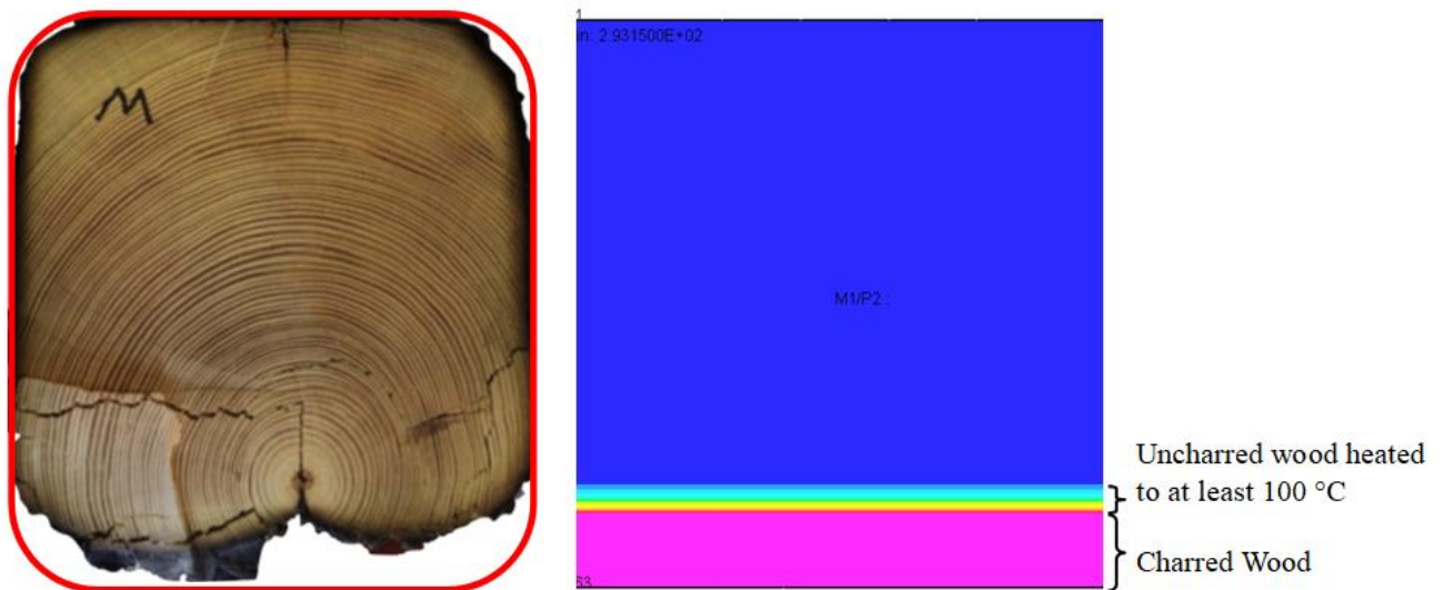
Figure 8.3 Comparison of the charred member and numerical model of a) the Glulam members and b) the heritage members
