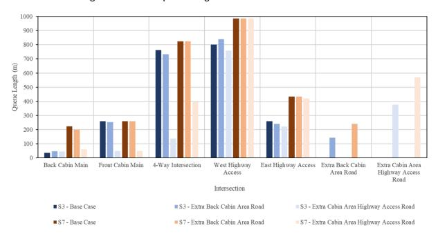
Fig. 10. Maximum queue lengths for main network intersections on the worst-case scenarios with additional egress roads
