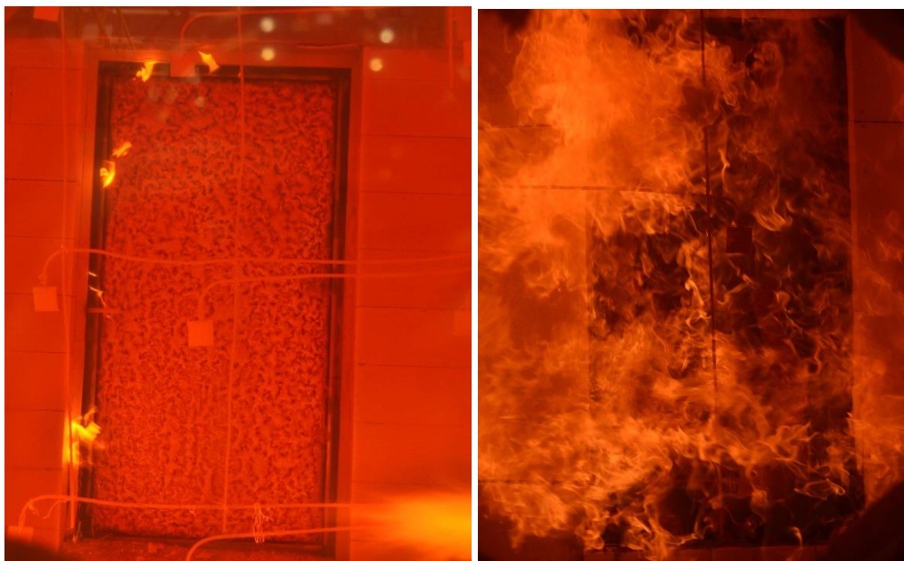
Fig. 2. View of the test sample inside the furnace left picture – aluminium doors with fire-rated glazing, right picture – wooden doors. Flame visible in the picture indicates combustion of the sample material (furnace burner is visible in the lower right corner of the left picture)
