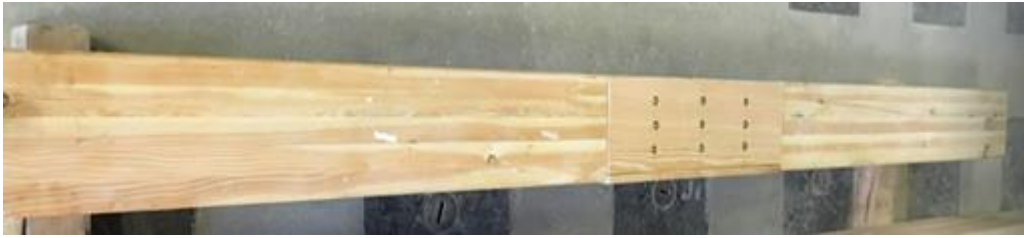
Fig. 3. Side of a repaired member.
