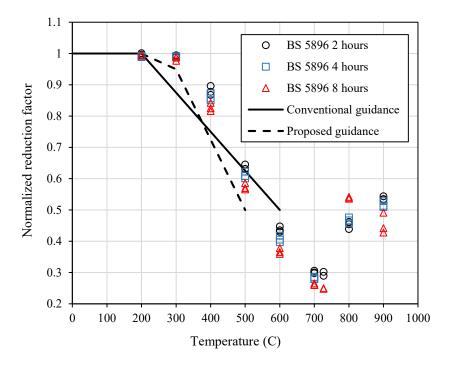
Figure 8. Contemporary prestressing steel strength reduction guidance.
