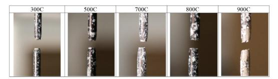
Figure 3. Fracture profiles for BS 5896 after two hours of heating.
