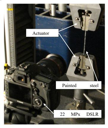
Figure 1. Loading apparatus with digital image correlation.
