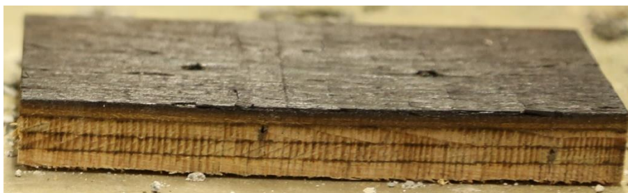
Fig. 12. Degradation process beginning on the timber, seen after removal of the iron plate
