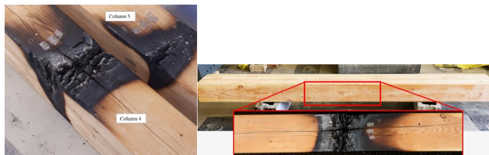
Figure 19. (left) Post-test condition of Columns 4 and 5 (right) post-fire cracking of Column 4 (note Columns 2 and 3 showed no signs of char damage)
