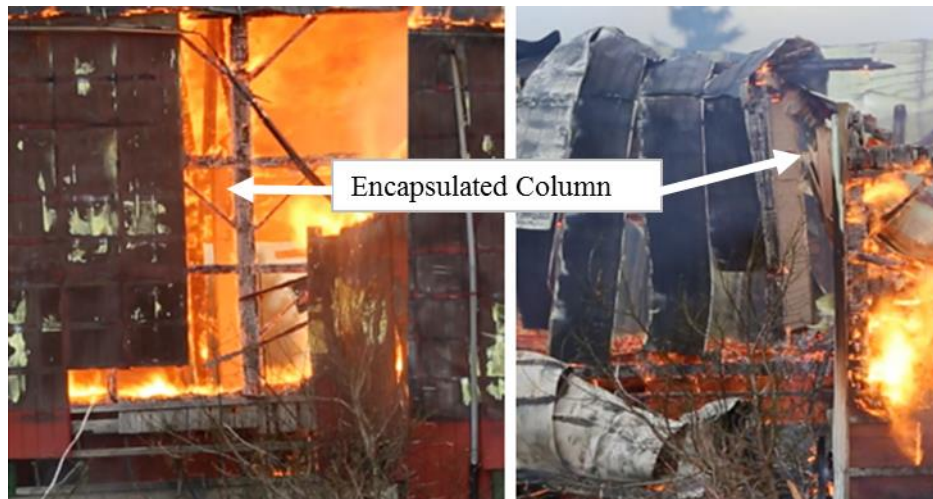
Figure 12. Images of Column 1 during field test (left) prior to structural collapse (right) post flashover event
