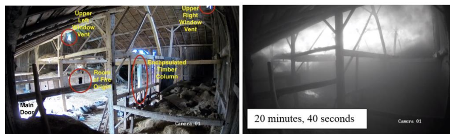
Figure 11. Pre heating view of compartment prior to fire ignition (left), atmosphere of compartment when fire spreads to column (right)
