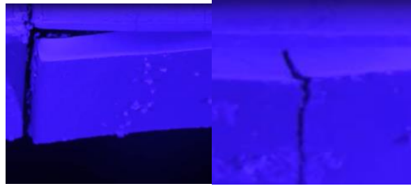
Figure 20. Delamination and cracking action of Gypsum Board at seam Column 2 during heating
