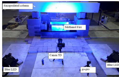
Figure 7. Specimen, apparatus, camera and LED light locations
