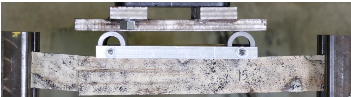
Fig. 6 Failure of an LVL beam, carved to the 10 mm damage state (carved area seen on the left-hand side of beam, bound by the split in the wood, and the support)
