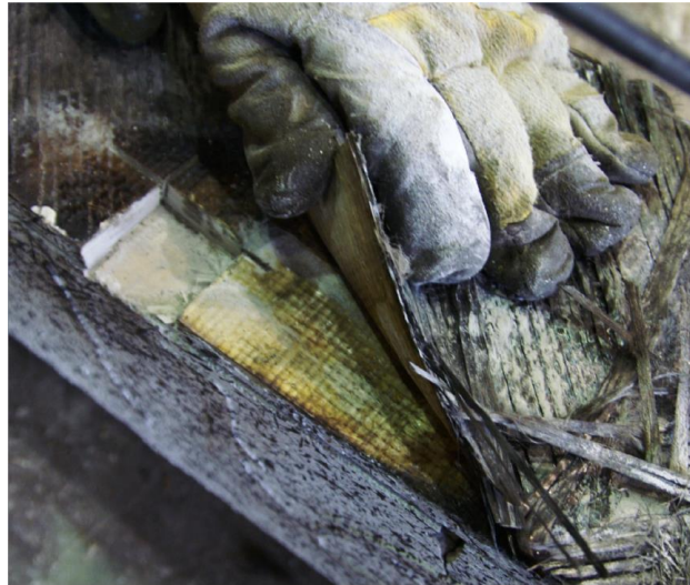
Fig. 23. Delaminated pyrolysis/char layer on GFRP base plate soffit.
