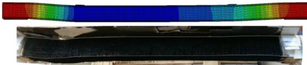
Fig. 13 Comparison of failure modes in numerical model (above) and experimental beam (below) for C3 where a shear region failure between the support outside the furnace and the load application point can be seen [5]
