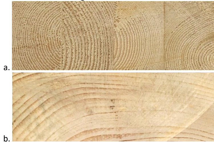
Fig. 4 Cross sections of showing the growth ring width of, a. contemporary Glulam and b. historic timber, from a building constructed in the 1840s
