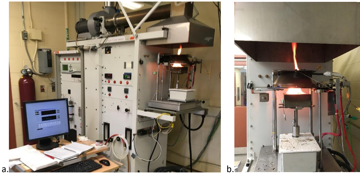
Fig. 9 The Calorimeter test setup, a. the entire apparatus and data collection system, and b. the cone heater and a sample being tested
