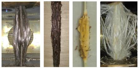
Figure 6. Samples after transient test: from left to right applied tensile loads are 75, 120, 160, and 200 kN, and failure temperatures are 547, 450, 340 and 160  $^{\circ}$ C respectively
