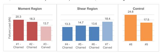
Figure 6. Comparison of the failure load of all beams damaged in the moment region, shear region, as well as the control beams
