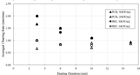
Figure 4: Averaged charring rates versus heating duration of all test specimens
