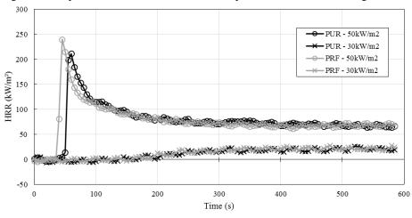
Figure 3: Sample heat release rate curves for samples with 10 minute heating duration
