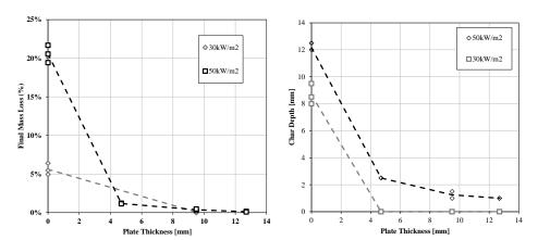
Figure 5: Plate thickness versus Char Depth and Mass Loss for 10 minute exposure
