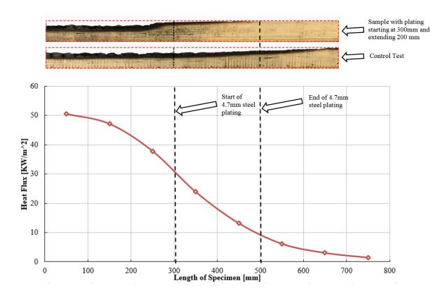
Figure 6: Char Depth of Sample Compared to Induced Heat Flux
