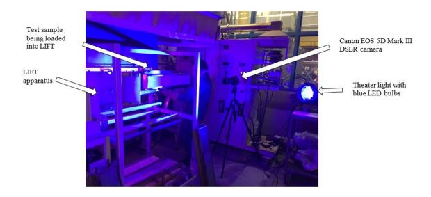
Figure 4: LIFT Apparatus and Imaging Setup in Carleton Campus Fire Lab
