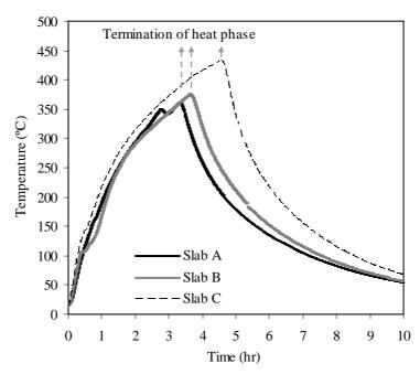
Figure 4 shows the average of the two PS tendon temperatures taken from thermocouples on the tendon at midspan for all three slabs; it is assumed that this would be the highest tendon temperature recorded anywhere, since this is where maximum tendon drape occurred and was the
