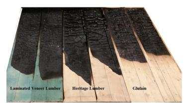
Figure 10. Timber Specimens after Heating.
