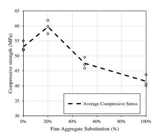
Figure 4: Cylinder compressive strength with fine aggregate substitution
