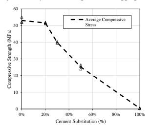
Figure 5: Cylinder compressive strength with recycled cement substitution
