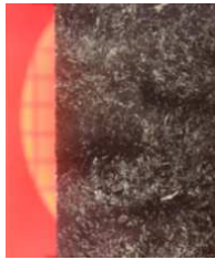
Figure 13: Cracking of tracking paint coating after exceeding its operational temperature limit.
