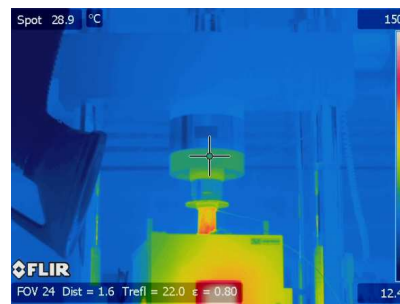
Figure 11: Thermal imaging of equipment frame at load cell showing negligible temperature rise outside furnace.
