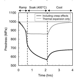
Figure 1: Stress variation in a restrained prestressing tendon due to localized heating (based on test data presented by MacLean et al. <sup>5</sup>)
