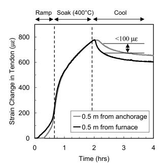
Figure 9: Recorded changes in tendon strain
