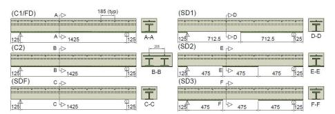
Fig. 1. Control and simulated damage specimens
