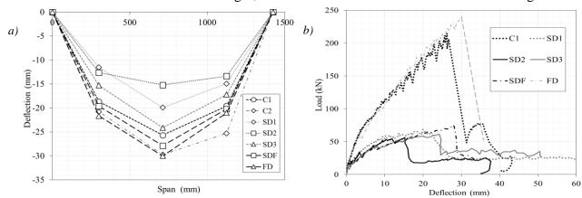
Fig. 4. a) Span-deflection at ultimate; b) Load-deflection responses of damaged strips
