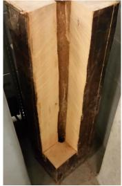
Figure 8. A heritage Beam (no. 3) after two strips were cut out to be tested under a controlled heat exposure. Note the hollowed core was traditionally added to prevent moisture accumulation.
