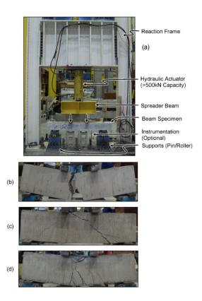
Fig. 1. (a) Test setup; Failure modes: (b) cracking moment; (c) shear failure; (d) flexural failure.
