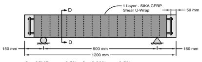
$f_c^{\prime}$  = 35MPa;  $\rho_1$  = 0.5%;  $\rho_1^{\prime}$  = 0.33%  $\rho_1$  = 0.5%; Failure Load (One Test)= 319.4 kN
