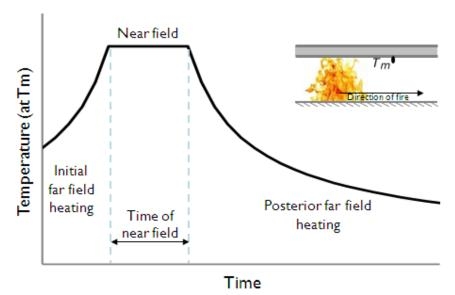
Figure 3 Gas temperature at an arbitrary point in a compartment (adapted from [11]).
