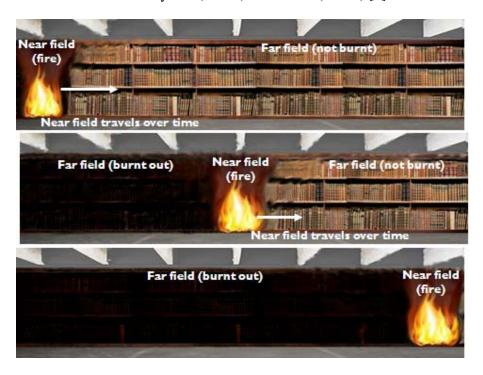
Figure 2 The travelling fires framework from ignition to burn out
