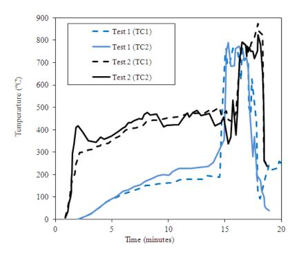
**Figure 1** The time and temperature history of the large compartment fire tests of the community hall (Test 1) and school (Test 2) [7]
