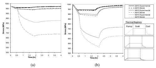
Figure 2: Stress versus time for (a) 11% heated length ratio and (b) 3% heated length ratio.
